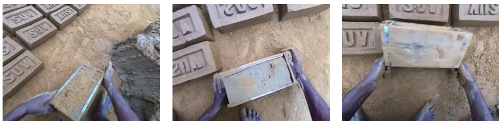
“How to pour clay mix from the brick mold on the ground?”
