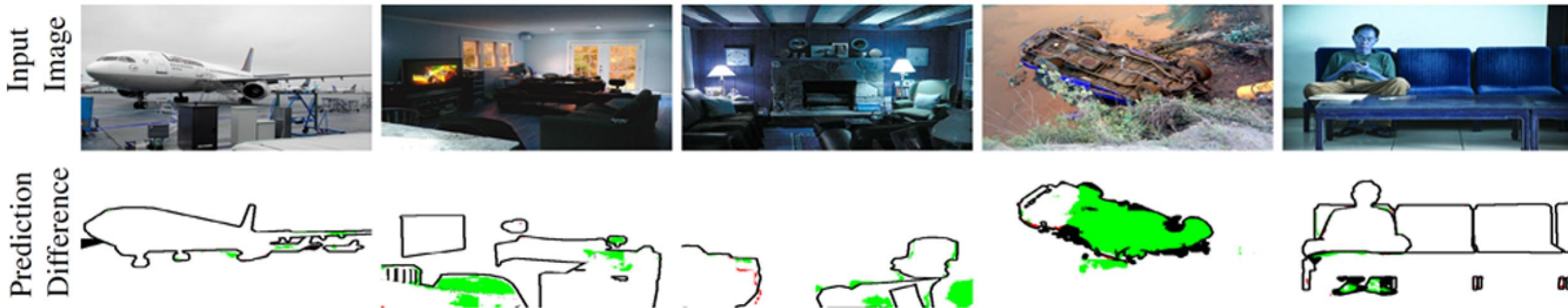
Figure 7. Difference in semantic segmentation mask predictions between LCTC and baseline transposed convolution using UNet [3] with ConvNeXt [4] encoder on PASCAL VOC2012 [5] image
