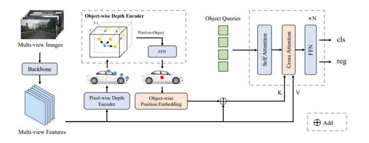
OPEN consists of the pixel-wise depth encoder (PDE), the object-wise depth encoder (ODE), and objectwise position embedding (OPE)
