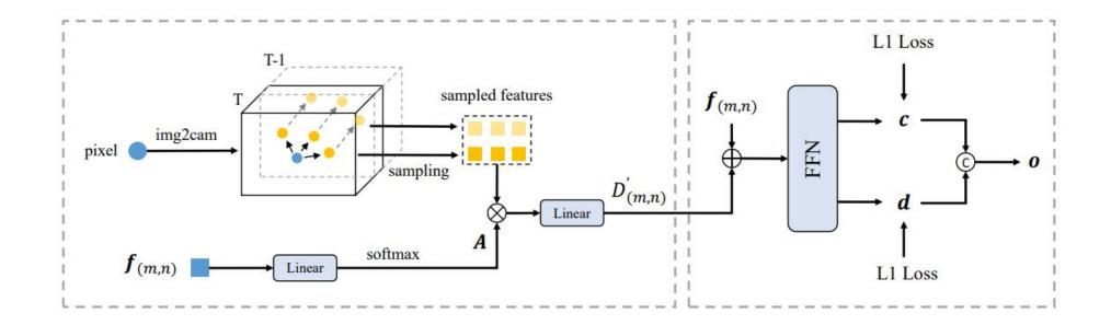
ODE predicts the object-wise depth based on pixel-wise depth information and streaming temporal fusion strategy in 3D camera space
