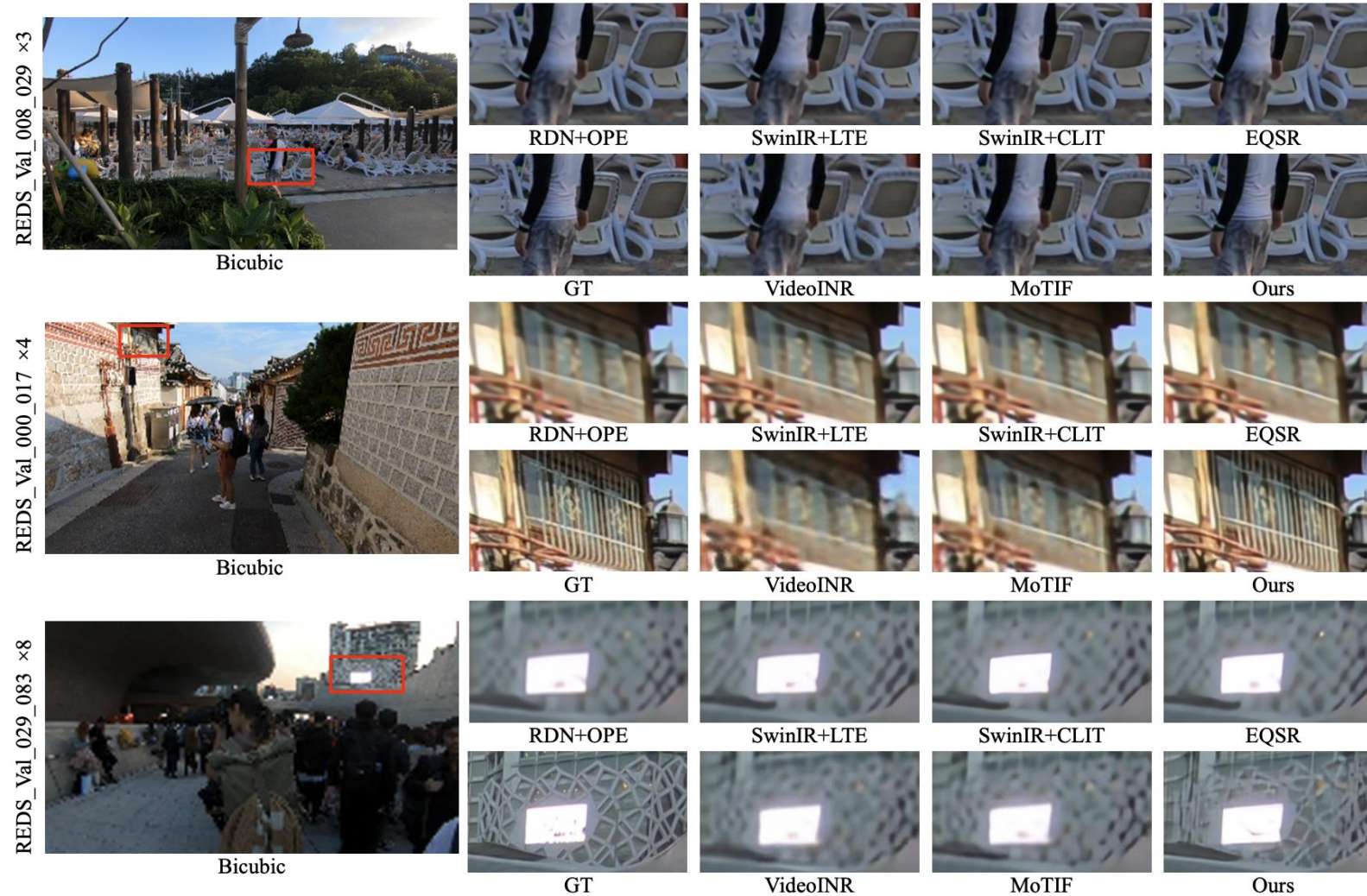
Fig. 4: Visual comparison for arbitrary-scale SR models on the REDS dataset. Please zoom in for better view.
